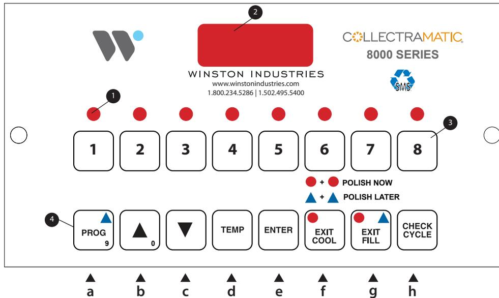
1. **LED Program Lamps** indicate which channel is selected when lit above that channel.
